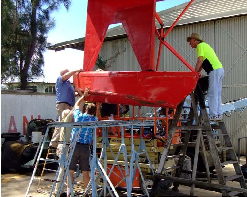
**Contact! The right-hand float is re-attached to the float pylon.
